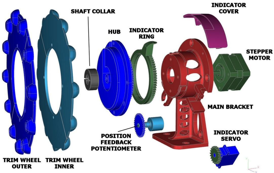
5. Fit the stepper motor to the Main Bracket. Make sure to rotate the stepper to bring the phase wires out through the ventilation holes in a position that suits your installation.
